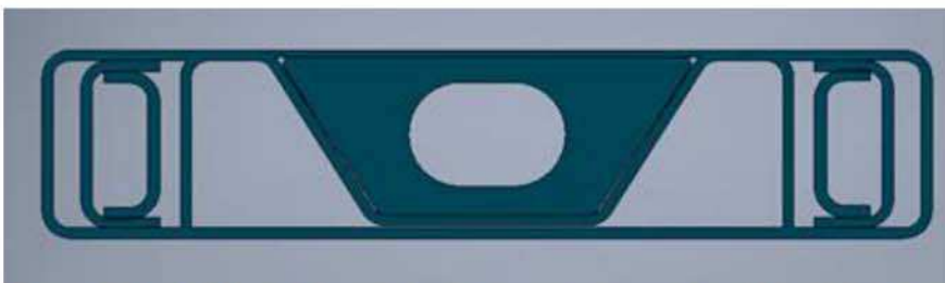
Figure 1.2: Old design frame for 92 tonmeter crane trucks with one pair of beam in cross section view. (SSAB, n.d.)
