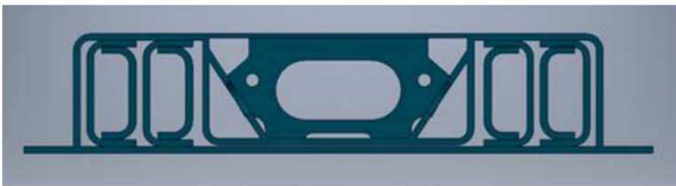
Figure 1.3: New design of crane truck central frame with double beam in cross section view. (SSAB, n.d)
