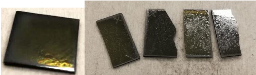
Sample with two sticking plates to each other and which separated while dicing.
