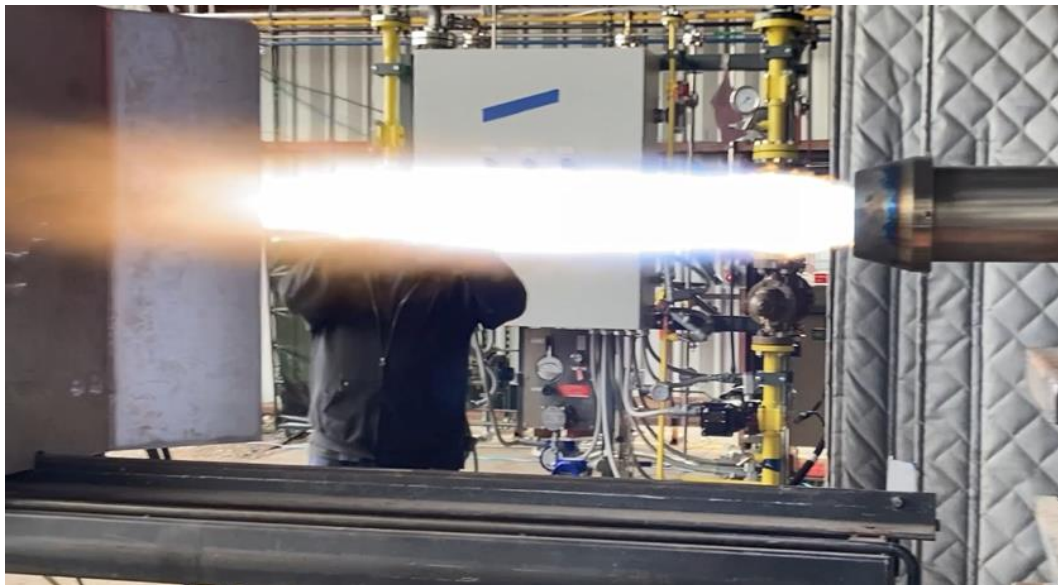
Figure 13 Stable flame during testing of the CoJet lance.
