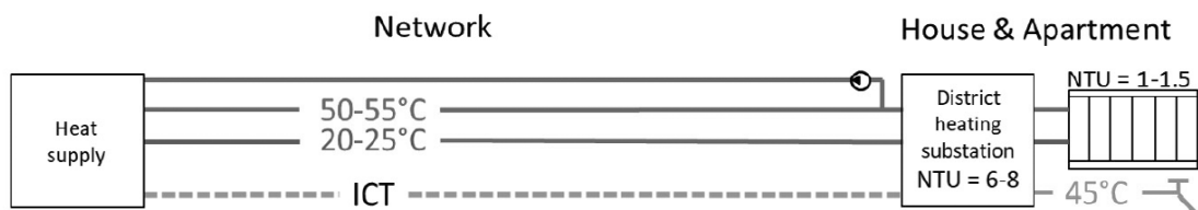
Figure 2. Sketch of two 3GDH systems currently in use and of the novel 4GDH which will be tested in Ranagård. The 86°C lines in the 3GDH denote the supply and the 47°C lines the return. The 55°C lines in the 3GDH denote domestic hot water. NTU denotes the number of heat transfer units and thermal lengths in substations and radiators. In the 4GDH the 50-55°C line denote the supply and the 20-25°C the return. Here the 4GDH, the domestic hot water has 45°C. ICT information and communication technology, the dotted line, is used in the 4GDH system for continuous measuring and control enabling improvements in locating temperature errors (Gadd & Werner 2013). Illustration by Averfalk & Werner (2018).
