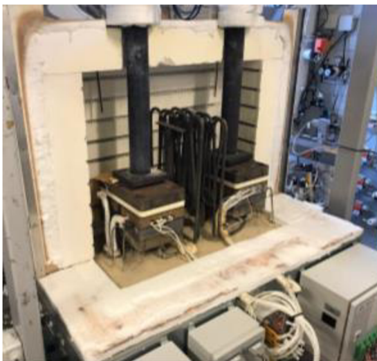
Figure 7. Dual-stack test station in VTT with installed E350 stacks and operating parameters
