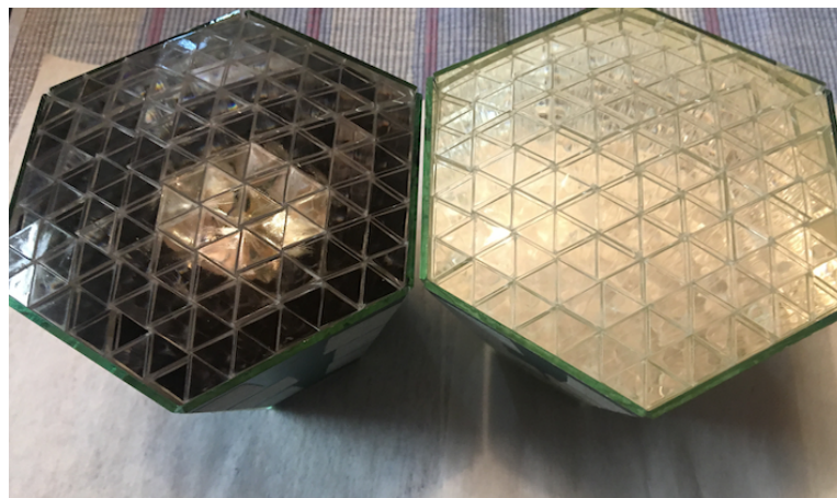
Figure 2. Side view of FC-concentrators (concentration = 3X) – left with an absorbing focal plane and right with a reflective focal plane. Consequently, the left concentrator absorbs all light within a wide acceptance angle hence its black appearance.
