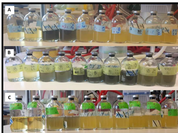
Figure 6. Anaerobic serum flasks with A, C. autoethanogenum ; B, C. carboxidivorans ; and C, C. ljungdahlii , after 10 days in PETC medium with, from right to left, 100, 100, 50, 50, 35, 35, 20, 20, 0 and 0 mM ammonia. Adapted from (VIII).
