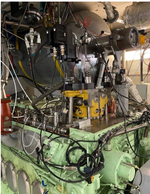
Figure 1: Wärtsilä W20DF test engine at Lund University.
