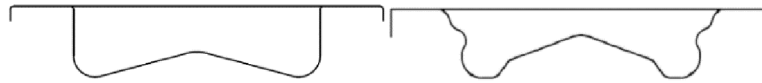
Figure 3: The piston bowl shape of two pistons. On the left is the modified straight wall piston. On the right is the standard production piston.
