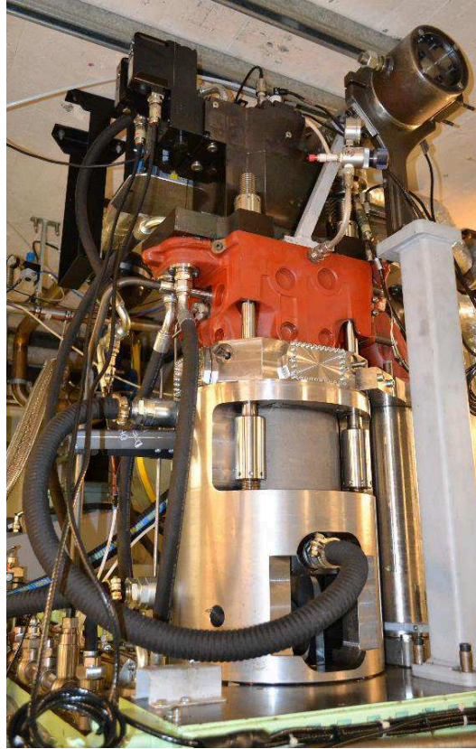
Figure 38: Wärtsilä 20 DF optical engine equipped with variable valve actuation.
