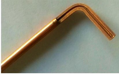
Fig. 3. Cut of the hollow conductor, showing that a 90° bend has no major impact on the inner diameter.
