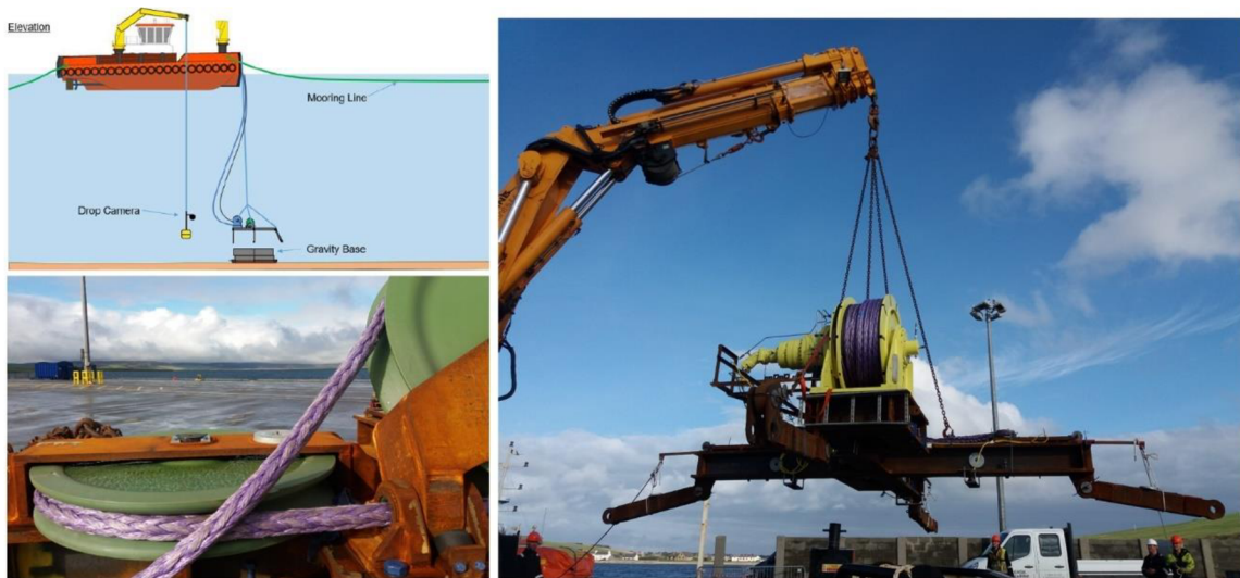
Figure 5. Anchor bracket with sub-sea winch and dynema tether.
