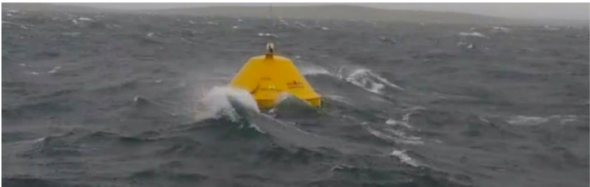
Figure 10 C3 WEC operating in waves up to 4m in detuned survival mode
