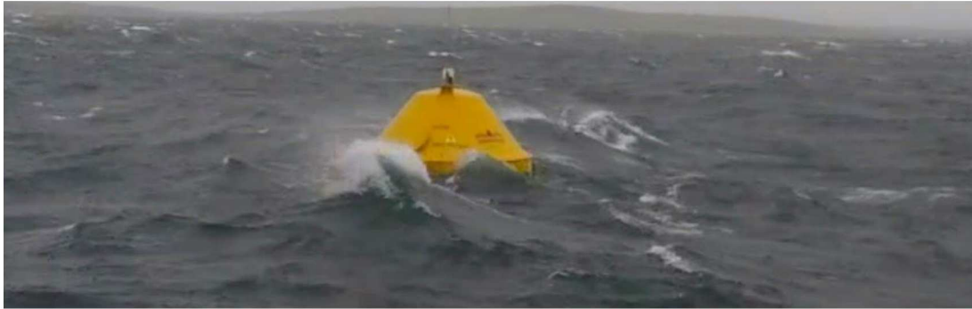
Figure 20 C3 operating in survival mode, 2.05m significant wave height, Scapa Flow, Orkney
