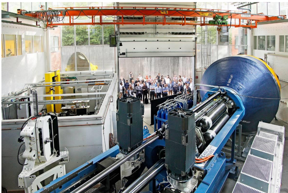
Figure 2 Stage 3 WEC in CorPower dry Hardware-in-the-loop testing facility, Stockholm (Sweden)
