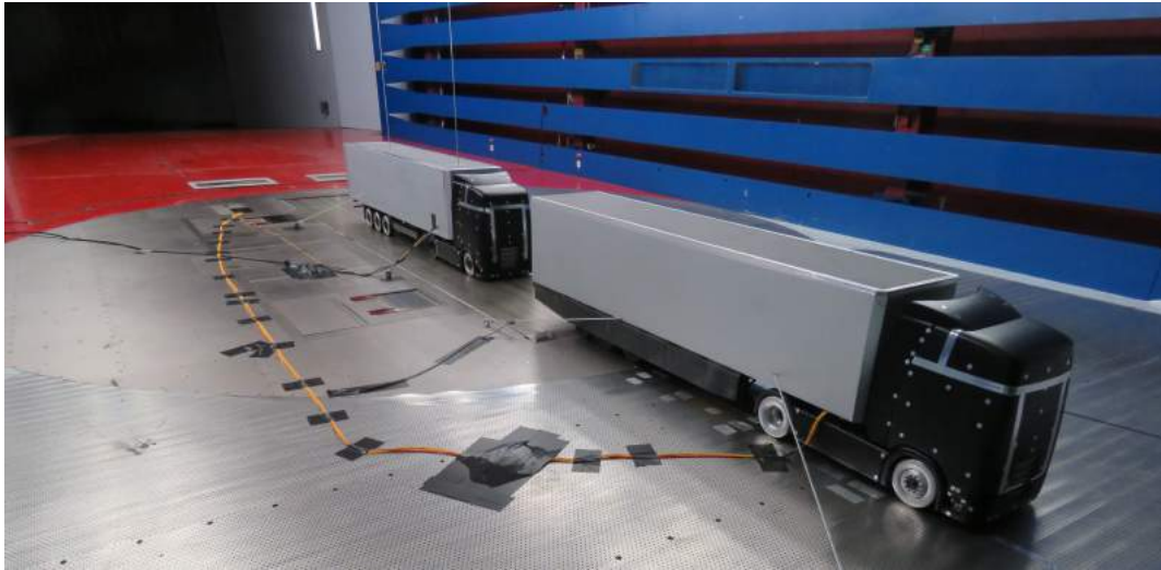
(a) Leading truck is the dummy model, and the trailing truck is the measurement model.
