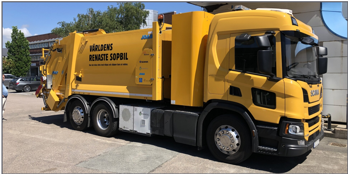
Figure 1.1 A PEMFC refuse truck operational in Gothenburg referred as Albert. [5]
