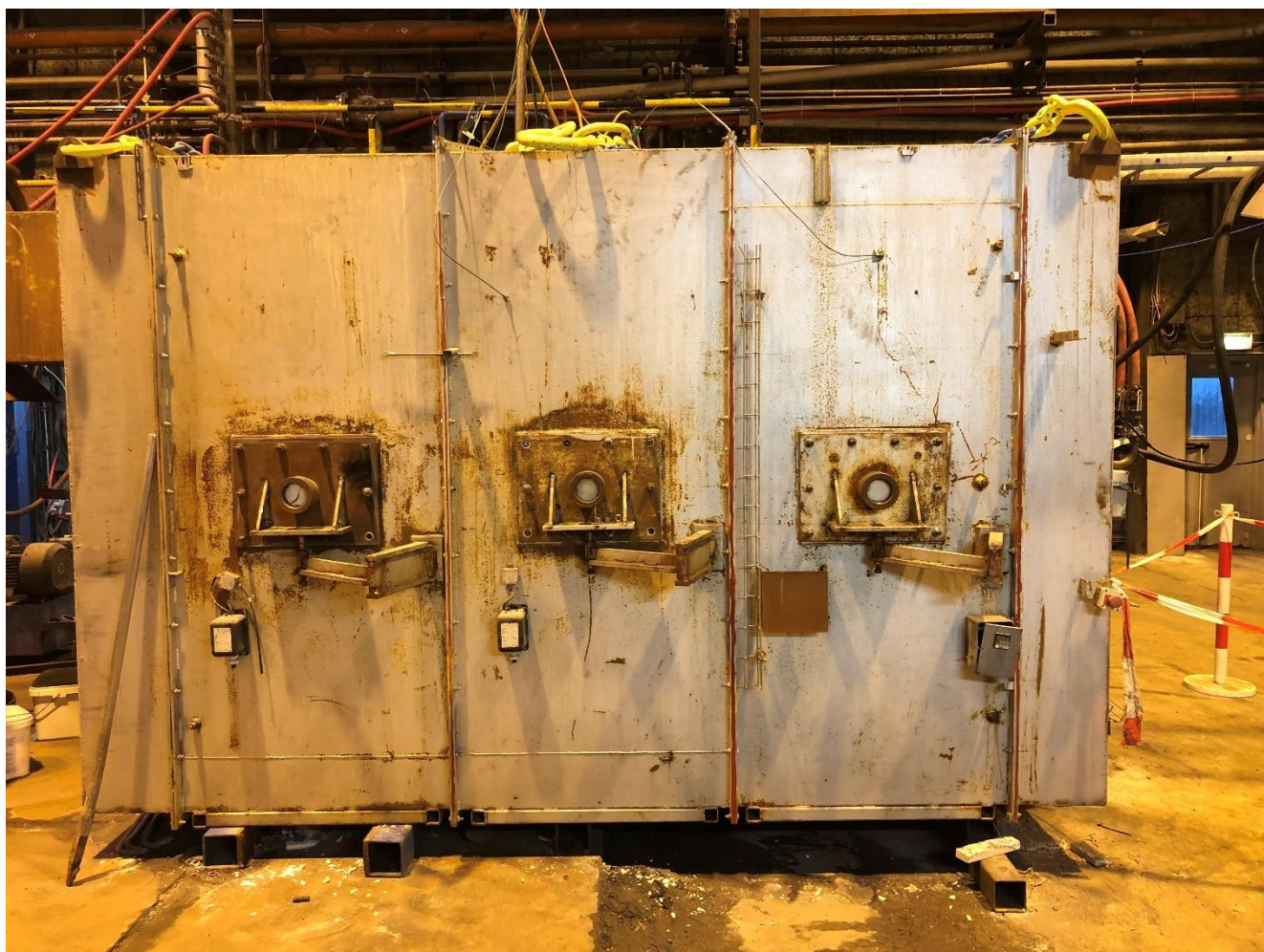
Figure 1 Trial furnace at Scanarc, seen from the side with three inspection hatches
