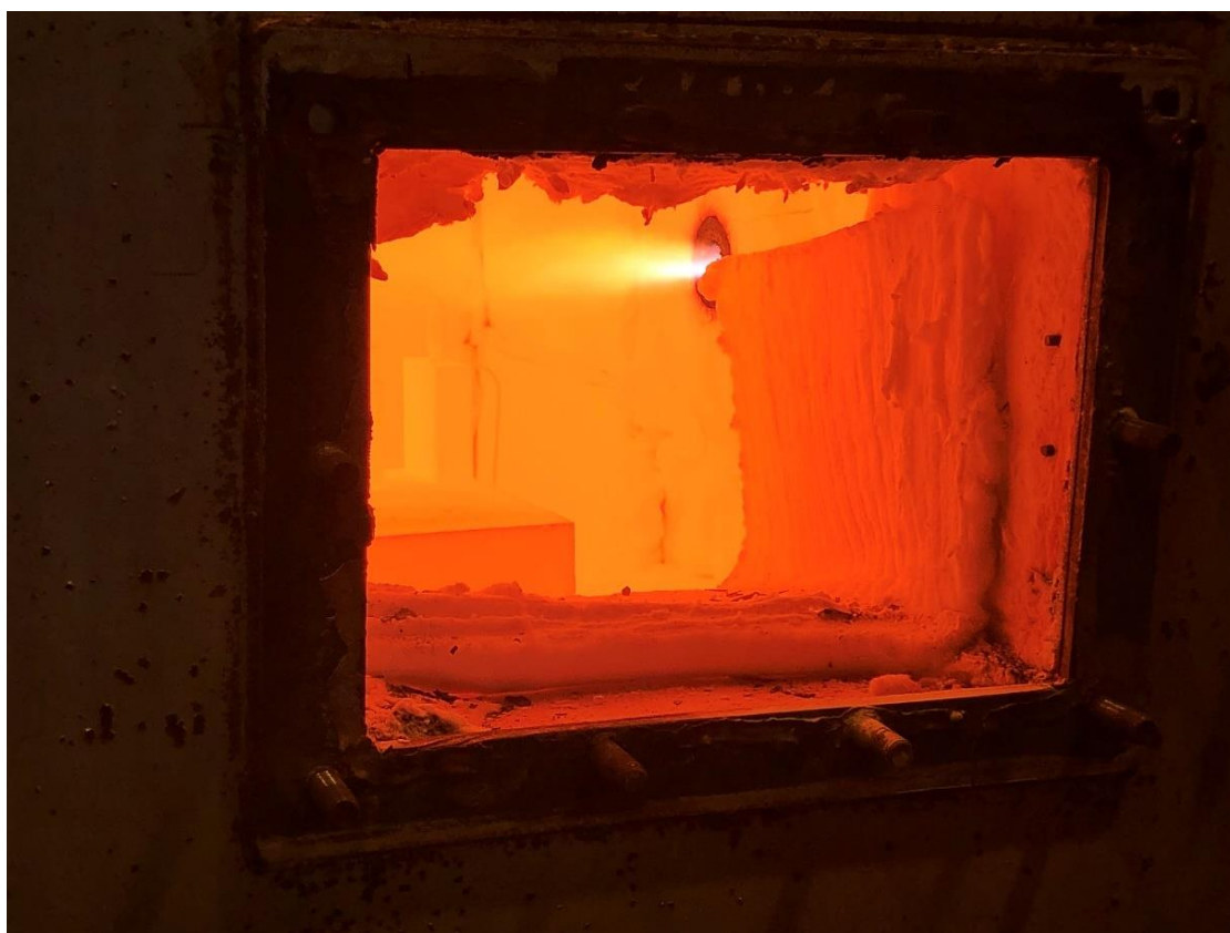
Figure 5 Plasma torch during heat up phase
