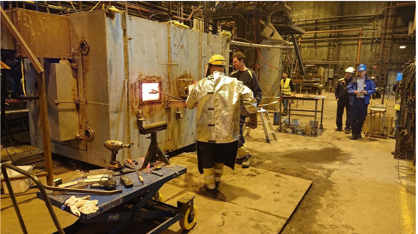
Figure 6 Unloading of steel samples during the trials from the test furnace.
