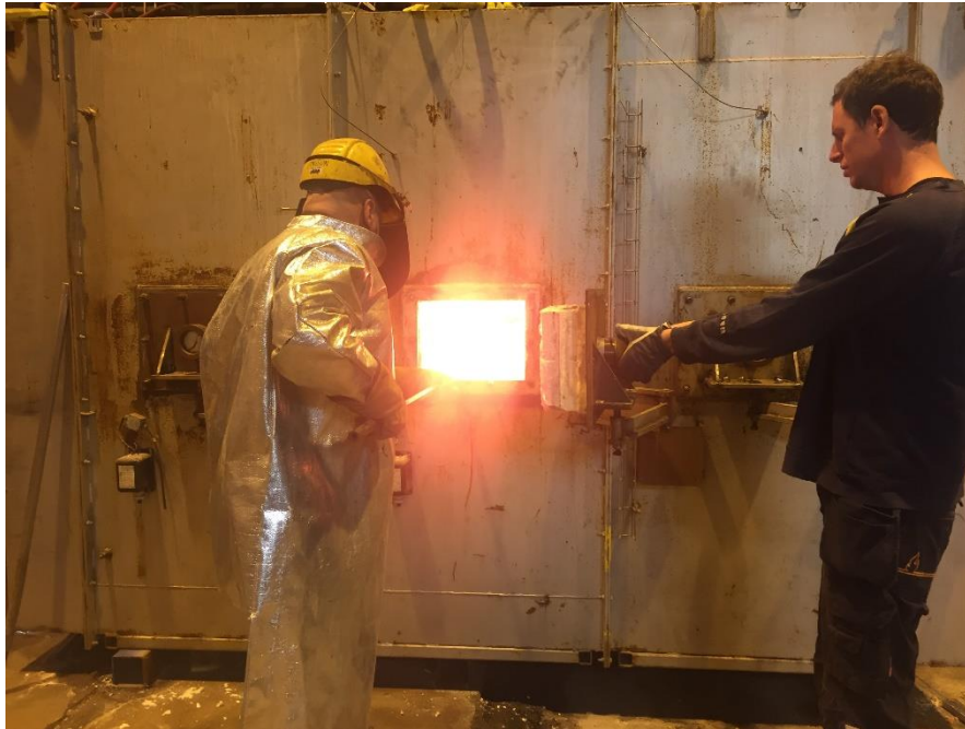
Fig. 3. Loading the steel samples through furnace's windows.
