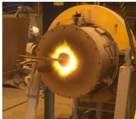
Fig. 27. Test configuration of plasma generator from ScanArc AB together with rotary batch kiln from Cemena Research [55].
