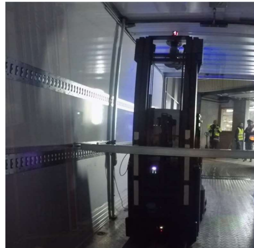
The Flexi Bar is back in start position when the AGV reverses
