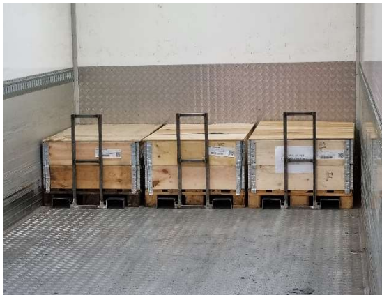
The L-frames are placed in the first section of three pallets in one layer
