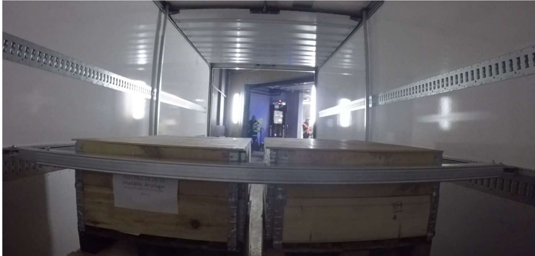
The second section are loaded, and the Flexi Bar blocks the upper layer in forward direction
