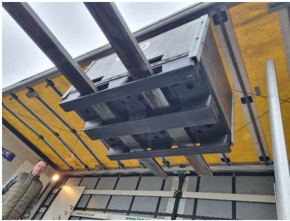
Some paint remains on the plastic pallet after the inclining test
