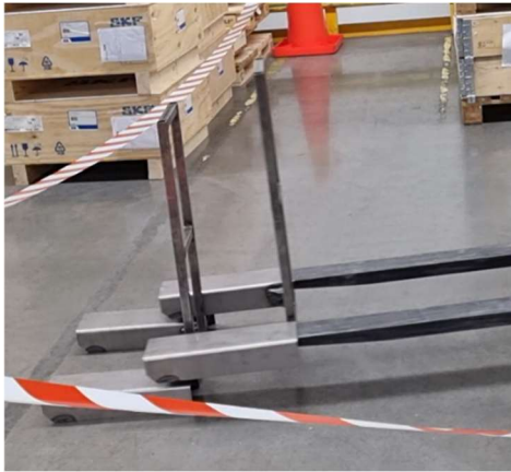
The L-frame is picked up by the forklift
