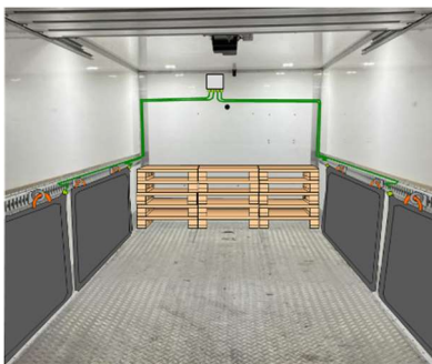
The dunnage bags are hanging in the shoring rails and connected to manifold system
