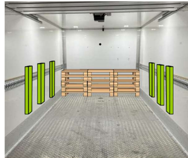
The cargo hold is ready for loading and the Moving Bars are retracted
