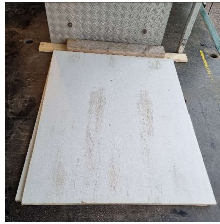
Traces of wear on the painted laminate after the inclining test
