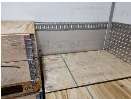
The second layer is forward blocked in forward direction by the L-frame
