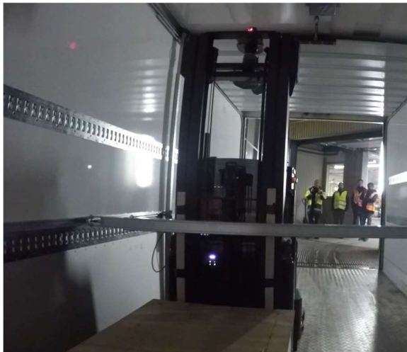
One pallet in the first section is loaded and the AGV push the Flexi Bar in forward direction
