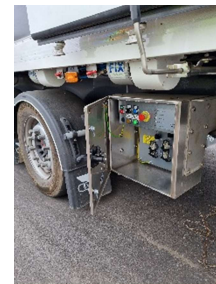
Control cabinet on the trailer for the FIX Truck-Safe system
