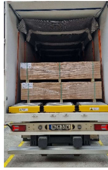
Cargo loaded and straps begins to be tensioned
