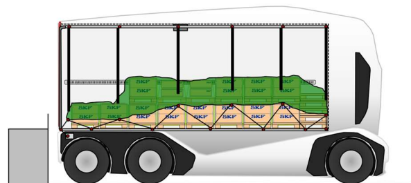
The tarpaulin is tensioned down against the cargo
