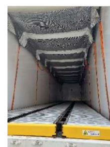
Moving floor in the semi-trailer and tarpaulin in start position
