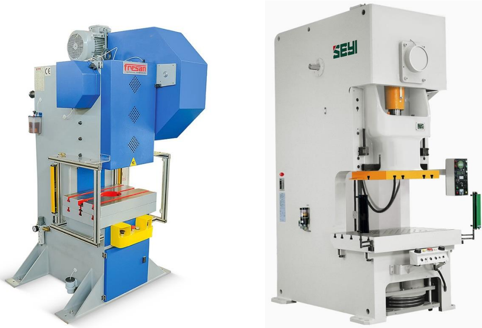
Figure 12 Mechanical eccentric press (left) and C-frame mechanical press (right).
