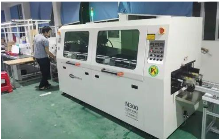
Figure 29 An automatic wave soldering machine for lead-free soldering of printed circuit boards with 300mm size from Shenzhen Jaguar Automation Equipment Co. Ltd
