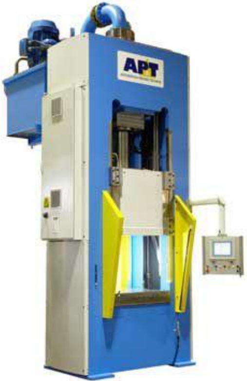
Figure 13 Hydraulic stamping press. Hydraulic cylinder on top of die holder.
