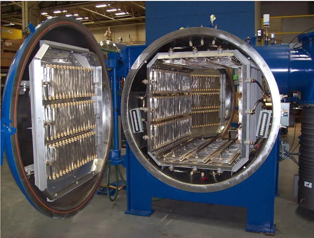
Figure 27 The appearance of a batch VB furnace for aluminium [39].
