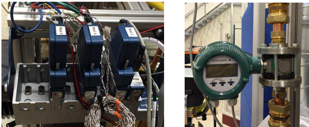
Figure 61 Chassis and data loggers (left) and magnetic flow meter (right).
