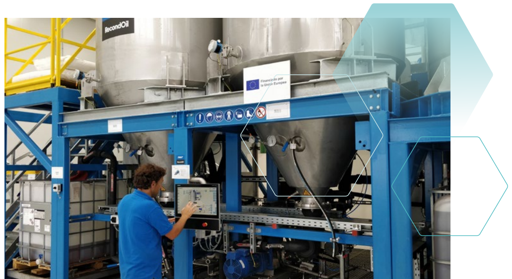
Figure 9. Project SKFOAAS – processing plant for reconditioning industrial lubricants using a double separation technology to remove all contaminants from used oils and return it to a clean, usable and high-grade product, thereby avoiding the disposal of the used oil.
