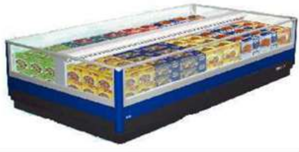
Figure 2-2 Open remote horizontal island for frozen products (category RHF4 according to EN ISO 23953), with 7 m 2 TDA, operating in temperature class L1 (-18°C to -15°C), using R404a as refrigerant, with a product life of 9 years.
