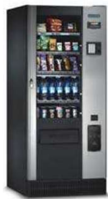
Figure 2-5 Spiral vending machine, with a net volume of 750 litres, operating in temperature class M2 (-1°C to 7°C), using R134a as refrigerant, with a product life of 8.5 years. Plug-in.
