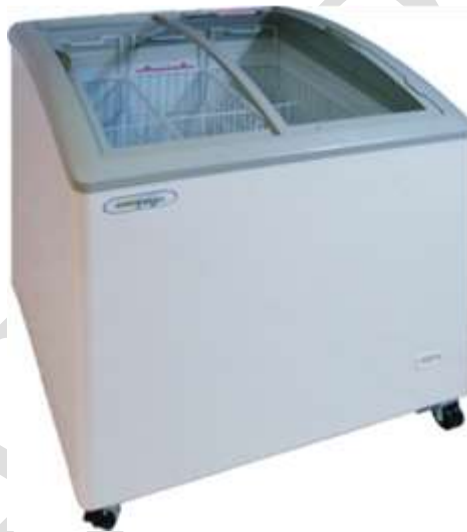
Figure 2-4 Packaged horizontal ice cream freezer with lids (category IHF6 according to EN ISO 23953), with a net volume of 291 litres, operating in temperature class L1 (-18°C to -15°C), using R507 as refrigerant, with a product life of 8 years. Plug-in.
