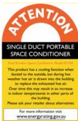
Figure 5: Proposed label designs for single duct air conditioners in Australia in 2009 64 . Text on the label: "This product has a cooling function when ducted to the outside, but during hot weather hot air is drawn into the building to replace the exhausted hot air. Over time this may result in an increase in indoor temperatures in other parts of the building. Please ask your retailer about alternatives."
